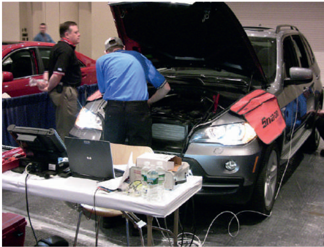
Figure 1.99 Bodywork protection in use during repairs
